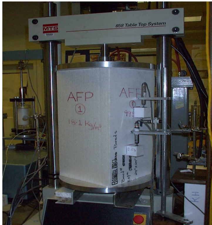
Photo 2. Creep test with hydraulic loading system on a 300 mm x 300 mm x 600 mm geofabric at 30% compressive strength
