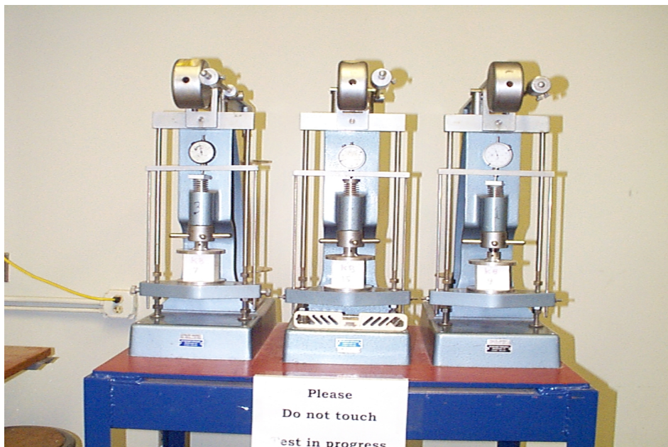
Photo 1. Creep tests with rear loading cantilever frames
