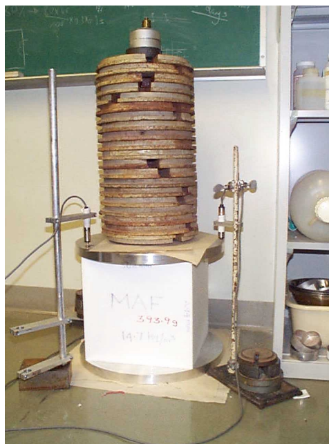
Photo 3. Creep test with dead loading on a 300 mm cube geofabric block at 30% compressive strength
